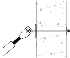
Tilt Up Wall with Thru Bolt
